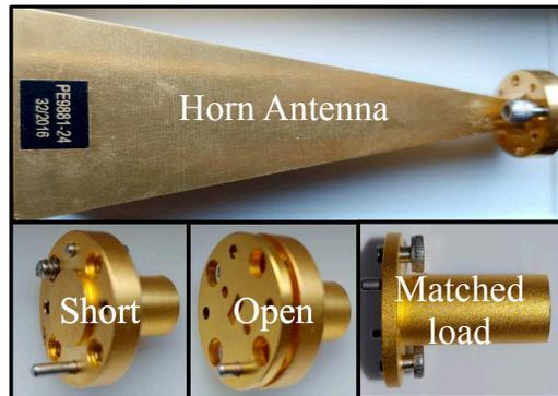
**Figure 5:** Horn antenna converted to the short and open-circuited antenna using a calibration short with and without the quarter-wavelength shim, respectively. The matched load offers an impedance match for the horn antenna.
